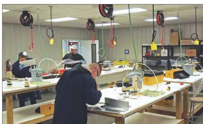
Above left —The Leland Unlimited Hydroplane Race Team has loaned a hydroplane to North Idaho College for composites technology students to splash and modify to instructor Trevor Budge's specifications. Above —In the layup, or clean, room, students learn infusion. The gray tanks are resin traps that prevent resin from entering the vacuum system. Each table has drops for air, electrical, and vacuum. Left —The first class in the Aerospace Composites Technology program gathers outside the hangar facility at the Coeur d'Alene Airport, in Hayden, Idaho.
