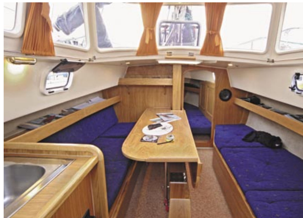
The table covers the centreboard case and lowers to form a double berth. Ballast is encapsulated in the bilge
