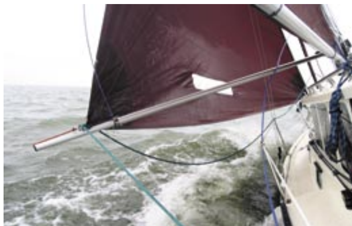
An uphaul and outhaul line on the pole allow accurate setting of the genoa
