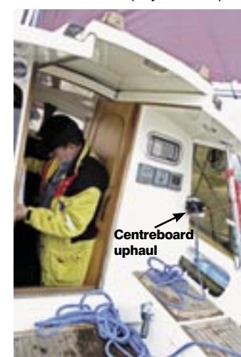
Extra shelter: protection is afforded by the overhanging roof of the deck saloon, plus a side screen. A Spinlock PX controls the main centreboard's uphaul
