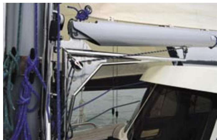
Limited space below the boom calls for an unusual kicking strap. It's tensioned and secured when the sail is hoisted; not adjusted under way
